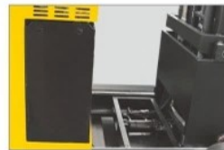
Oil tube inside of the mast with clean wire communications
